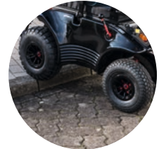
Obstacle climbing ability up to 110 mm
