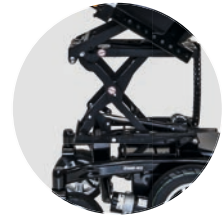
Electric seat tilt with optional 300 mm scissor lift
